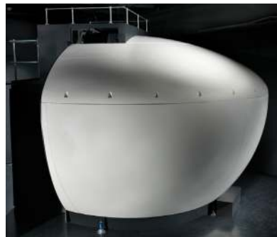
Cross-cockpit collimated display system. Fully integrated displays for enhanced side-by-side cockpit training.
