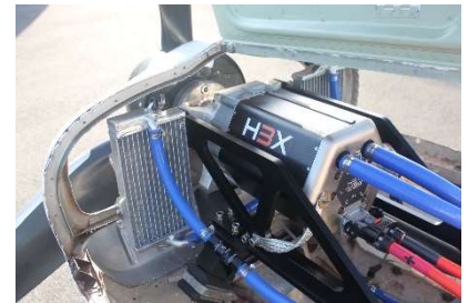
Photo | Clyde's hydrogen electric engine. Image supplied Stralis.
